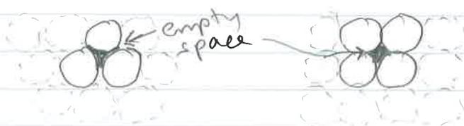
If we placed an atom on top of these holes we create an empty pocket called an interstitial void.
